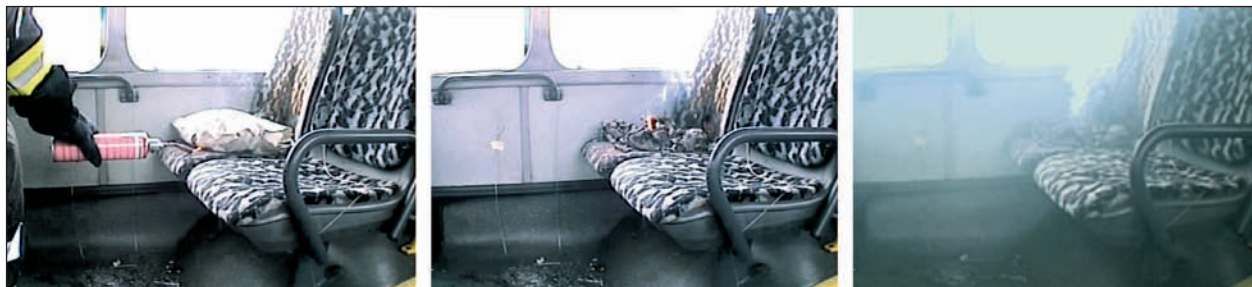
Fig. 55: Large scale test, the second try (ignition, burnt paper, remains)
