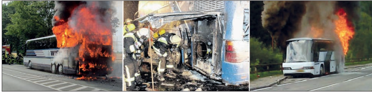
Fig. 1: Fires in the engine compartment of buses [FELGENTRÄGER 2012]
