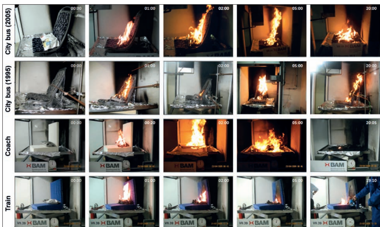
Fig. 37: Passenger seats in calorimeter tests
