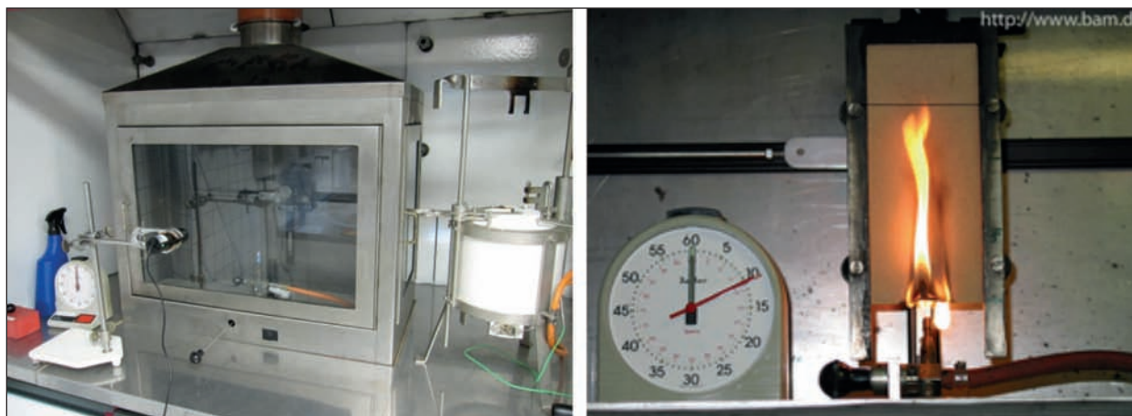
Fig. 34: Single-flame Source Test at BAM
