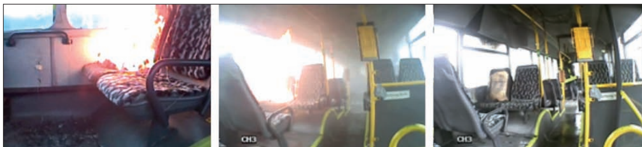
Fig. 56: Large scale test, the third try (burning clothes, burning seat, remains)
