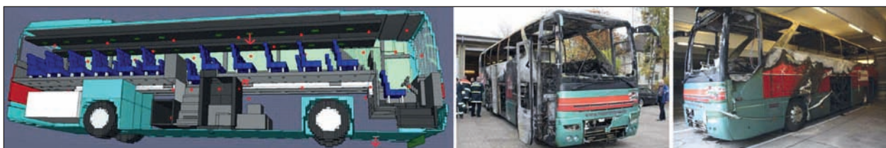
Fig. 22: Second bus model and its original from the Hannover bus fire [BUHRS 2008]
