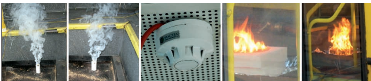
Fig. 41: Smoke cartridge (left), smoke detector (middle) and PU foam (right)
