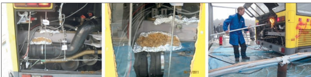
Fig. 47: Fire and extinguishing tests in the engine compartment
