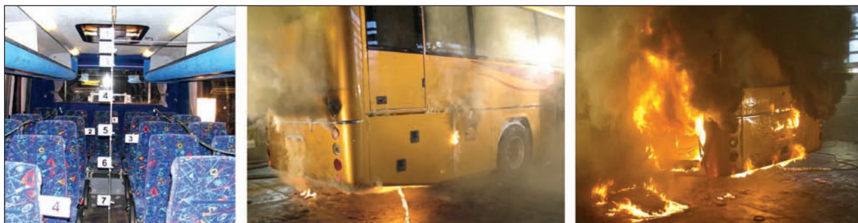
Fig. 58: Cuttings from the real scale bus fire test from SP [HAMMARSTRÖM 2008]
