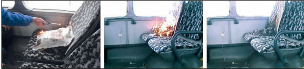
Fig. 54: Large scale test, the first try (ignition, burning paper, remains)
