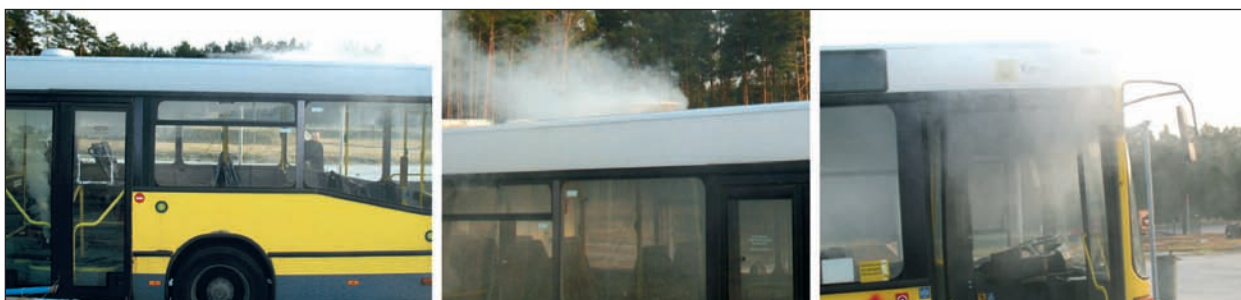
Fig. 43: Smoke spread test in the passenger cabin
