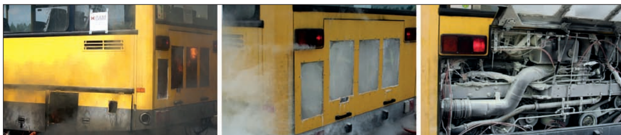
Fig. 52: Engine compartment before, while and after the fire suppression in fire series IIc
