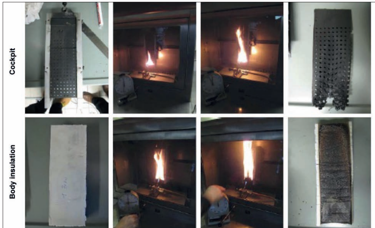
Fig. 35: Bus materials in Single-flame Source Test
