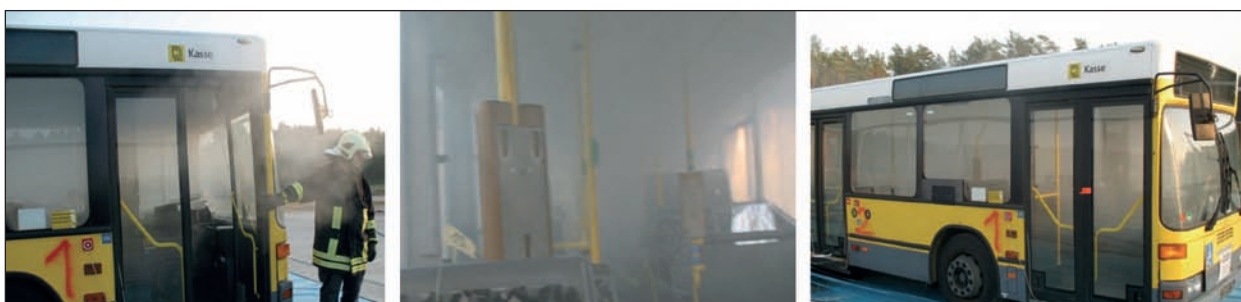
Fig. 40: Smoke spread test in the passenger cabin
