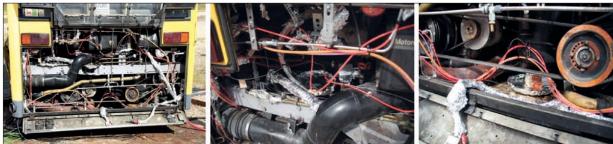
Fig. 50: Engine compartment prepared for pool fire tests
