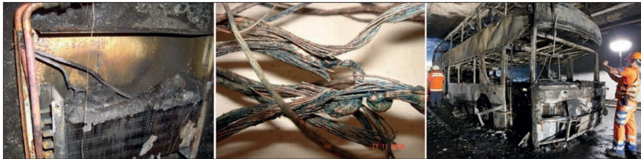
Fig. 2: Bus fires caused by defects in electrical components [BUHRS 2008]
