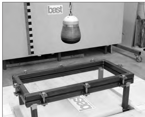
Fig. 9: Phantom head drop test – impact configuration
