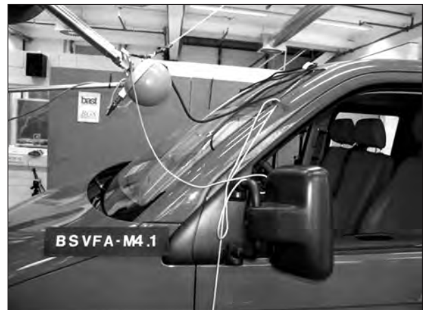
Fig. 12: Test setup with 35° impact angle
