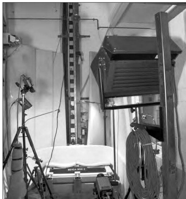
Fig. 1: Drop test with adult headform – test setup
