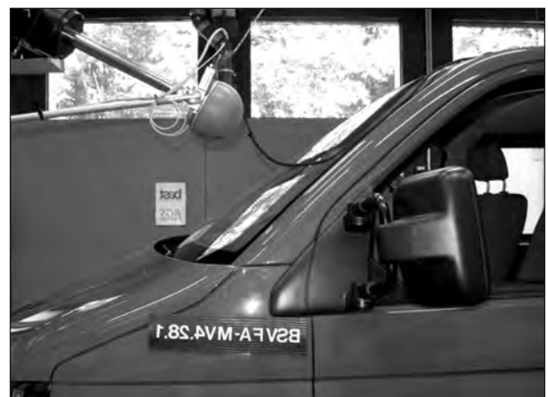
Fig. 13: Test setup with 28° impact angle
