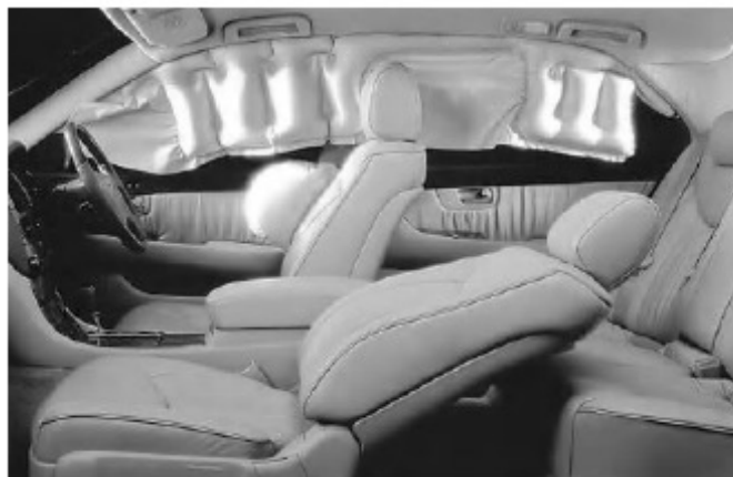
Figure 17. Restraint system for impact against a pole
