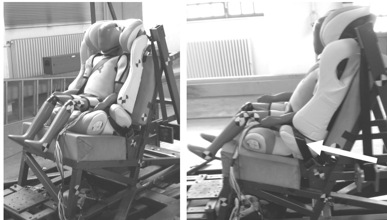
Figure 6: Sled test with group 2/3 CRS; Left: correct installation; Right: Installation with wrong belt guide
