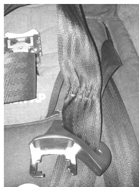
Figure 5: Belt marks caused by the CRS buckle
