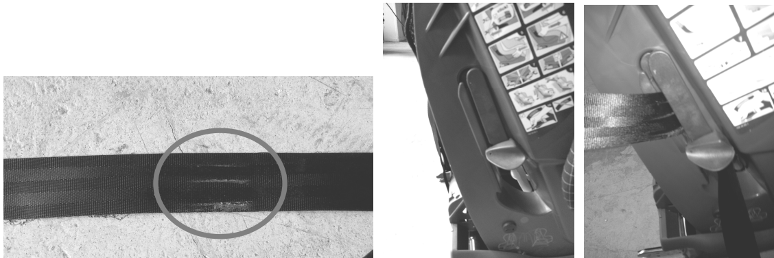
Figure 3: Belt abrasion marks from the CRS belt clamp
