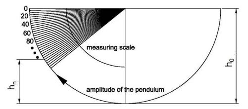
Figure 6: principle of the pendulum process
