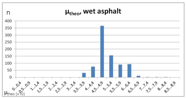
Figure 2: Theoretical friction coefficient calculated out of the measured SRT-values at the accident site
