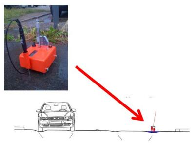
Picture 4: Measuring of the water depth
