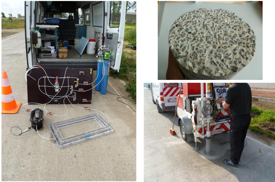
Figure 8 – Measurement of the photocatalytic efficiency on site (left) and in the laboratory, on cores taken from the site (right).
