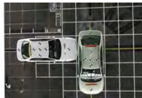
(b) 90-degree side impact, front and side-right
