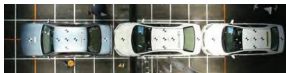
Figure 4. Multiple rear-end collision crash tests
