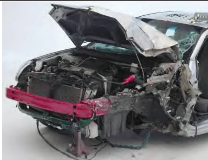
Figure 2. Pole test condition, 2007 Mitsubishi Galant
