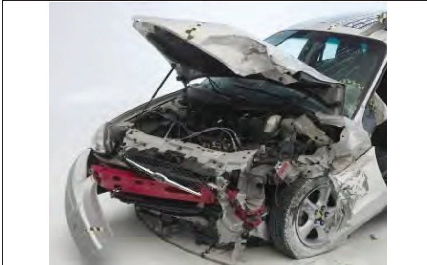
Figure 4. Vehicle-to-vehicle oblique test condition, 2002 Ford Taurus
