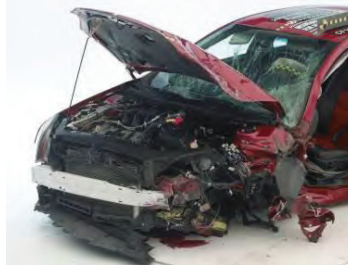
Figure 3. Vehicle-to-vehicle collinear test condition, 2008 Ford Fusion
