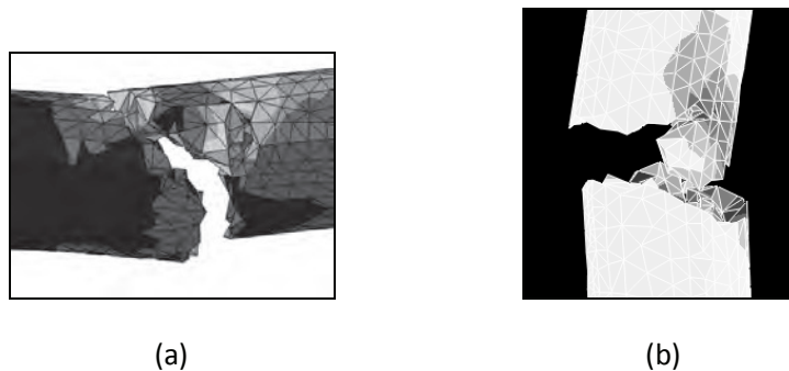
Figure 6 Simulation results for A-P impact direction for different cut-off stress (a) Oblique, 55 Mpa, Pendulum setup (b) Comminution, 45 Mpa, Cart setup
