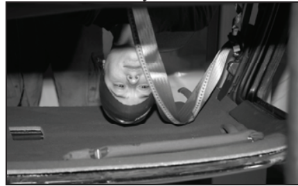
Series 6: Cinching Latch Plate with Slack
