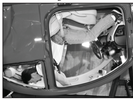
Series 7: Cinching Latch Plate with Slack in Pitched Vehicle
