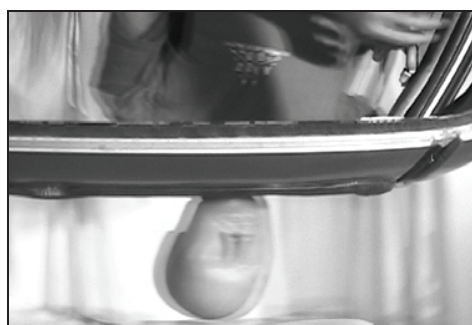
Figure 6. Test Series 9 ATD Dynamic Excursion
