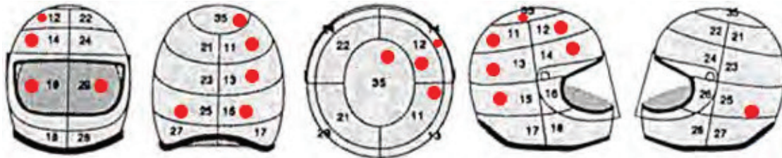
Figure 10 – Damaged zones of the helmet.
