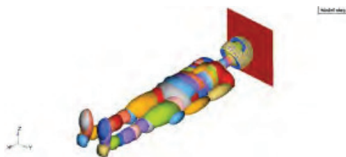
Figure 17 – Future simulations using anthropomorphous model Hybrid III.
