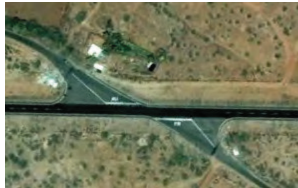
Figure 14. Intersections with Poor Road Alignments on the NH67 (Scene Diagram on the left) and NH47 Bypass (Google Earth Image on the right).
