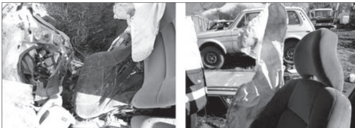
Figure 4: Case 2 – intrusion and deployed side airbags at driver's position
