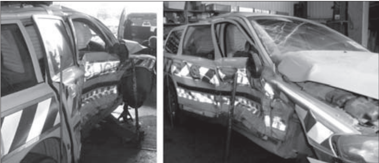
Figure 1: Case 1 – side impact damage
