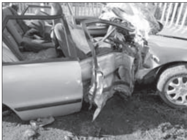
Figure 3: Case 2 – side impact damage
