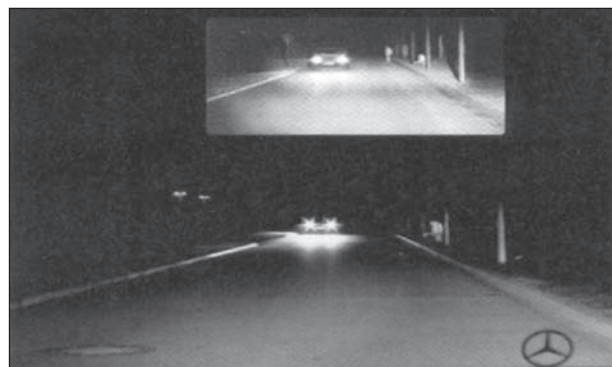
Fig. 13: Enhanced visual image system
