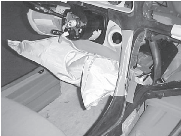
Fig. 1: Location of the inflated knee bag system
