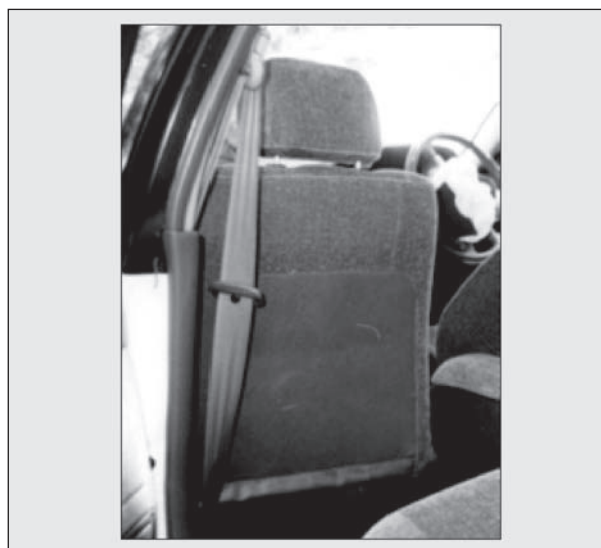
Fig. 1: Deformation of front seat (No. 2)
