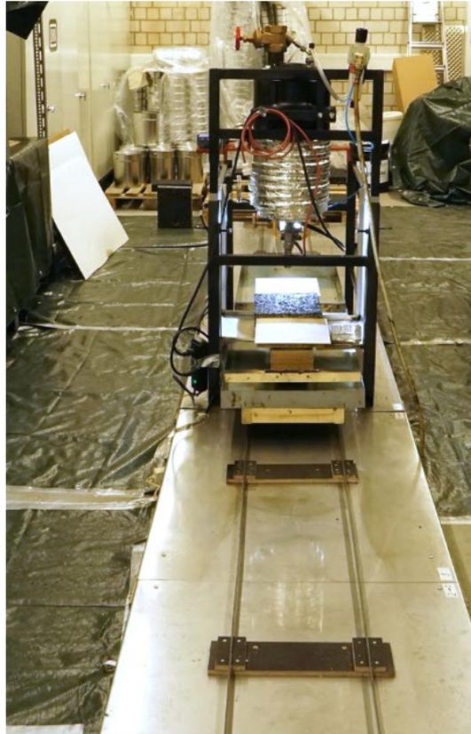
**Figure 1: Spraying plant for application of bitumen emulsion**
