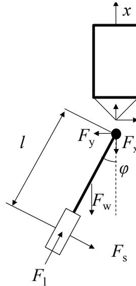
**Figure 1: Forces at the trailer coupling for a trailer at an articulation angle, with longitudinal wheel force  $F_l$ , lateral wheel force  $F_s$ , driving resistance  $F_w$ , shear force at the trailer coupling  $F_y$  and longitudinal force at the trailer coupling  $F_x$ . The figure shows the aforementioned unicycle model which assumes that both wheels are subject to equal driving forces.**
