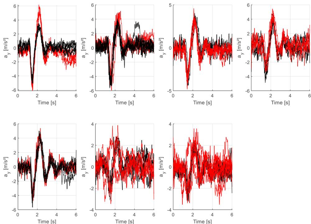
**Figure 12: Lateral acceleration in the trailer as a result of the defined steering impulse, at all speeds driven, example: Manufacturer A vehicle**
