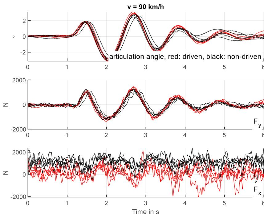
**Figure 3: Sample measurements (Manufacturer A vehicle) of articulation angle, shear force and longitudinal force in the drawbar at a driving speed of 90 km/h after a defined steering impulse according to ISO 9815 has been given.**
