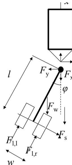
**Figure 2: Forces acting on the trailer coupling of an articulated trailer. As above, with additional left longitudinal force on wheel  $F_{l,l}$ , right longitudinal force on wheel  $F_{l,r}$  and track width  $w$ .**
