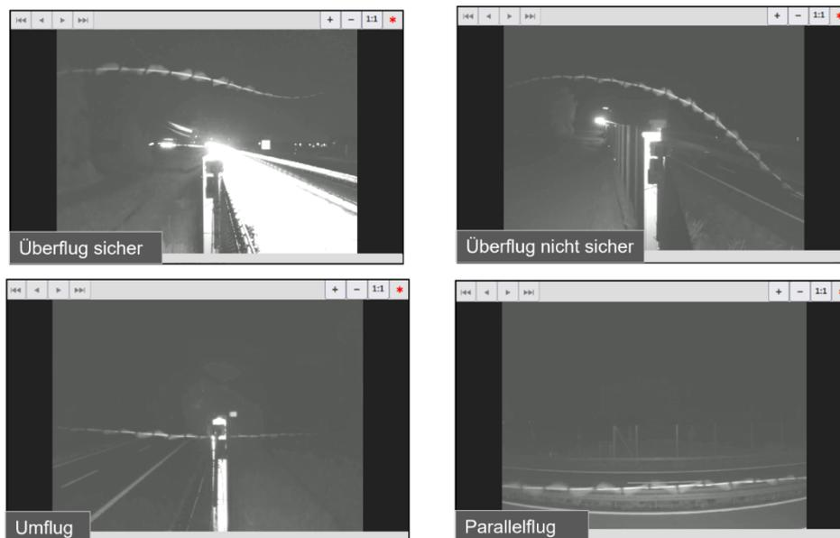
Figure 2-2: Examples of the observed behavioural categories recorded by the infrared cameras (composite images). Top left: a safe crossing over the crossing aid, top right: an unsafe flight over the crossing aid, bottom left: a flight around the end of the crossing aid, bottom right: a flight parallel to the crossing aid.
