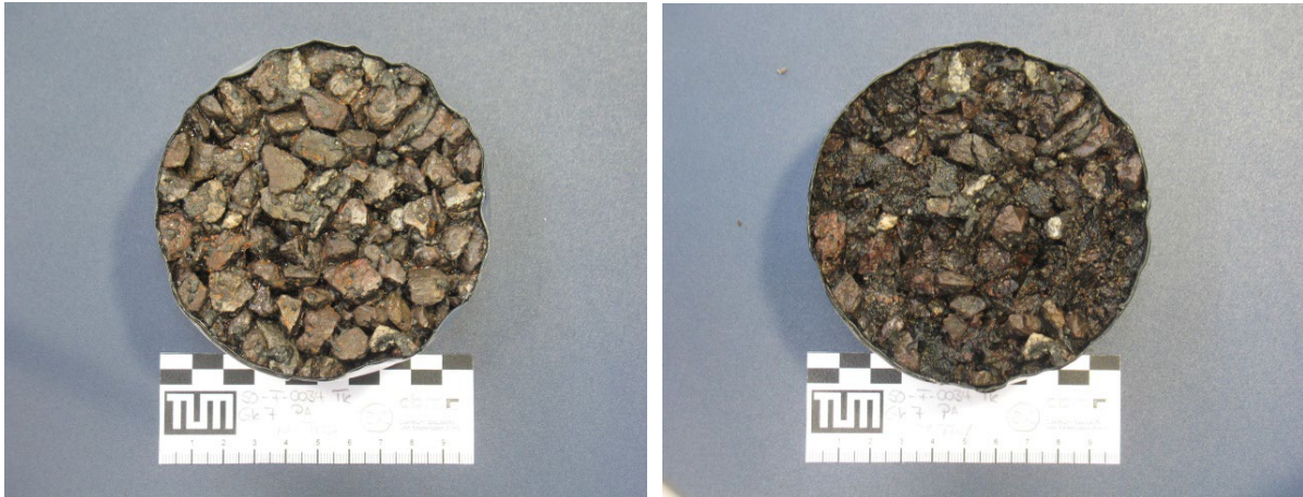
Figure 3 Test specimen of the porous asphalt (PA) with GK 7 before (left) and after (right) the 28 freeze-thaw cycles in the CDF asphalt test
