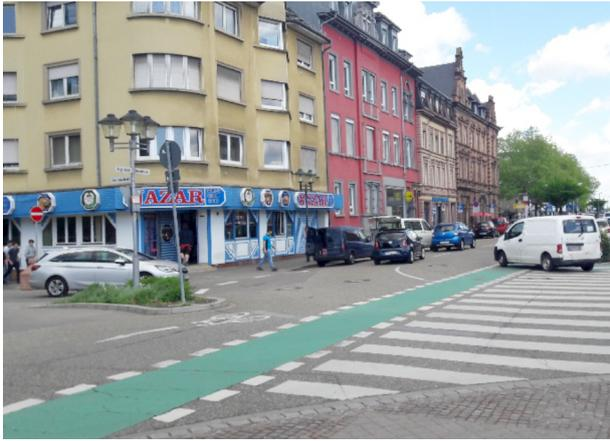
**Fig. 4: Continuous colour marking of cycling infrastructure (INOVAPLAN 2018)**
