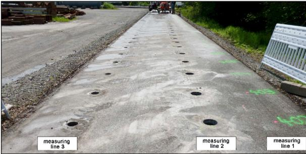
Fig. 3: Sampling the measuring lines of the 2,000 MHz radar antenna using drill cores in a 1-m-grid
