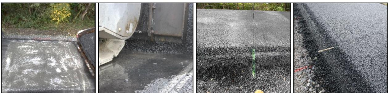
Fig. 2: Selection of artificially produced structural damages on the test track
