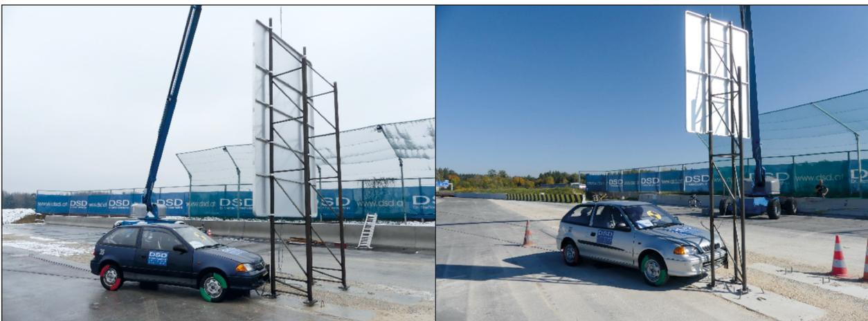
Fig. 2: Impact configuration “Gabelständer” 750 x 76 mm and “Trimast” 500 x 60 mm prior to the test
