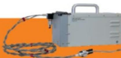
The High Concentration NPET derives from the basic and unique design of the NPET 3795, which allows you to bring laboratory-grade particle counting to your worksite. With similar design to instruments used in certification testing, the built-in catalytic stripper removes volatile particles to enable measurements of total solid particle emissions only.
