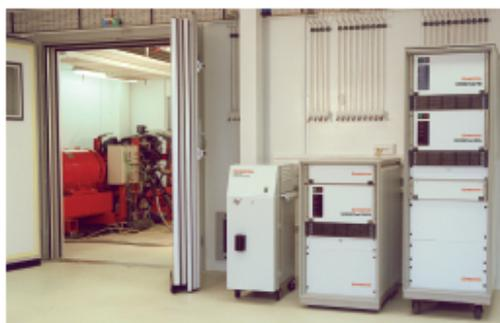
DMS500 shown with other ultra-fast Combustion analyzers (HC, NO<sub>x</sub>, CO & CO<sub>2</sub>)
