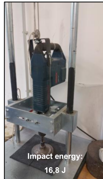
Image 3: Vibrating hammer B
