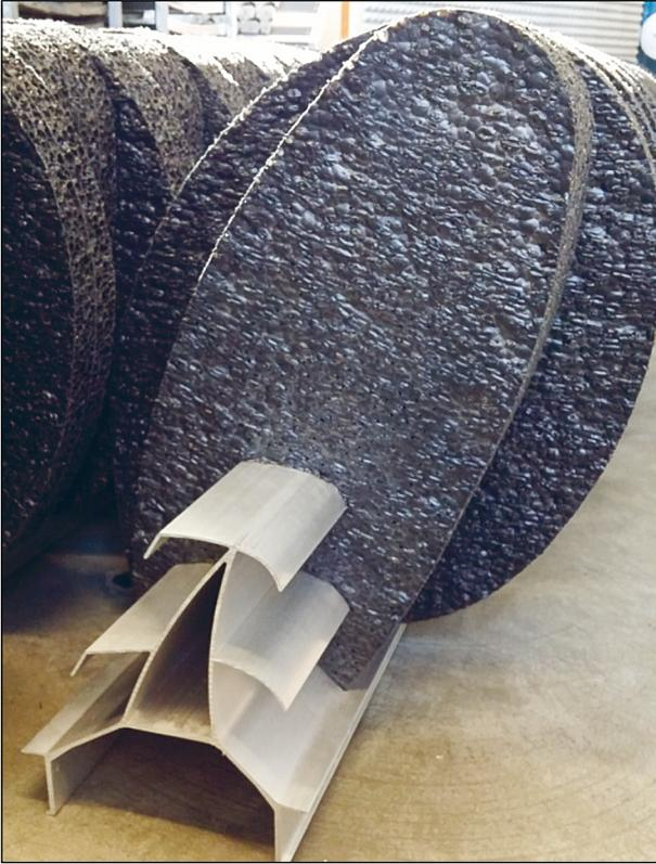
Fig. 1: Noise barrier add-on system under investigation
