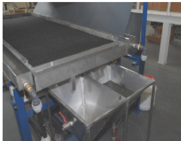
Figure 5: Test assembly for dirt transport, drain abilities and sound absorption.
