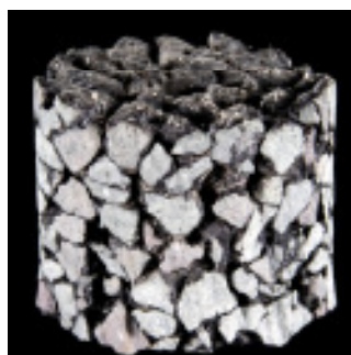
Figure 7: Computer tomographic picture of a porous asphalt sample.
