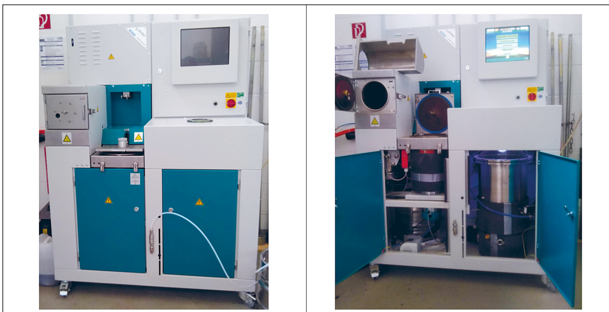
Fig. 2: Automatic extraction enclosure, suitable for the solvent OME at ISBS, with closed (left) and open (right) doors
