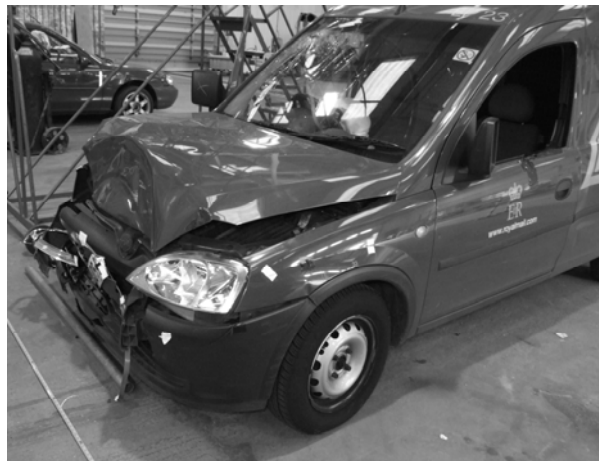
Figure 7. The damage to the Vauxhall Combo Van
