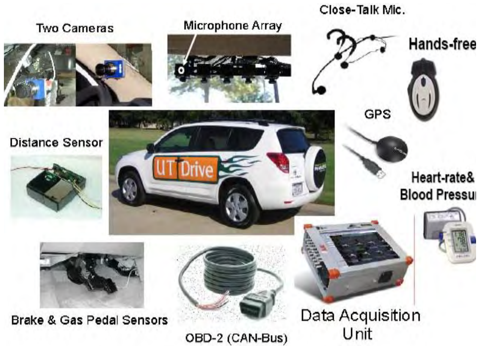
Figure 1. Data collection vehicle and incorporated sensors
