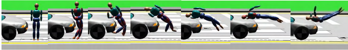
Figure 8. Car-to-pedestrian (2) real accident simulated on PC-Crash®
