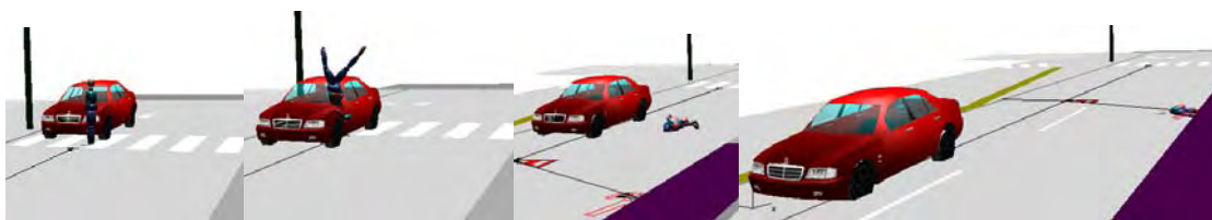
Figure 7. Car-to-pedestrian (1) real accident simulated on PC-Crash ®
