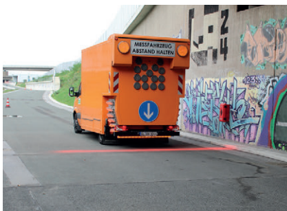
BAST's MEFA measurement vehicle in action on the duraBAST reference section for longitudinal evenness
