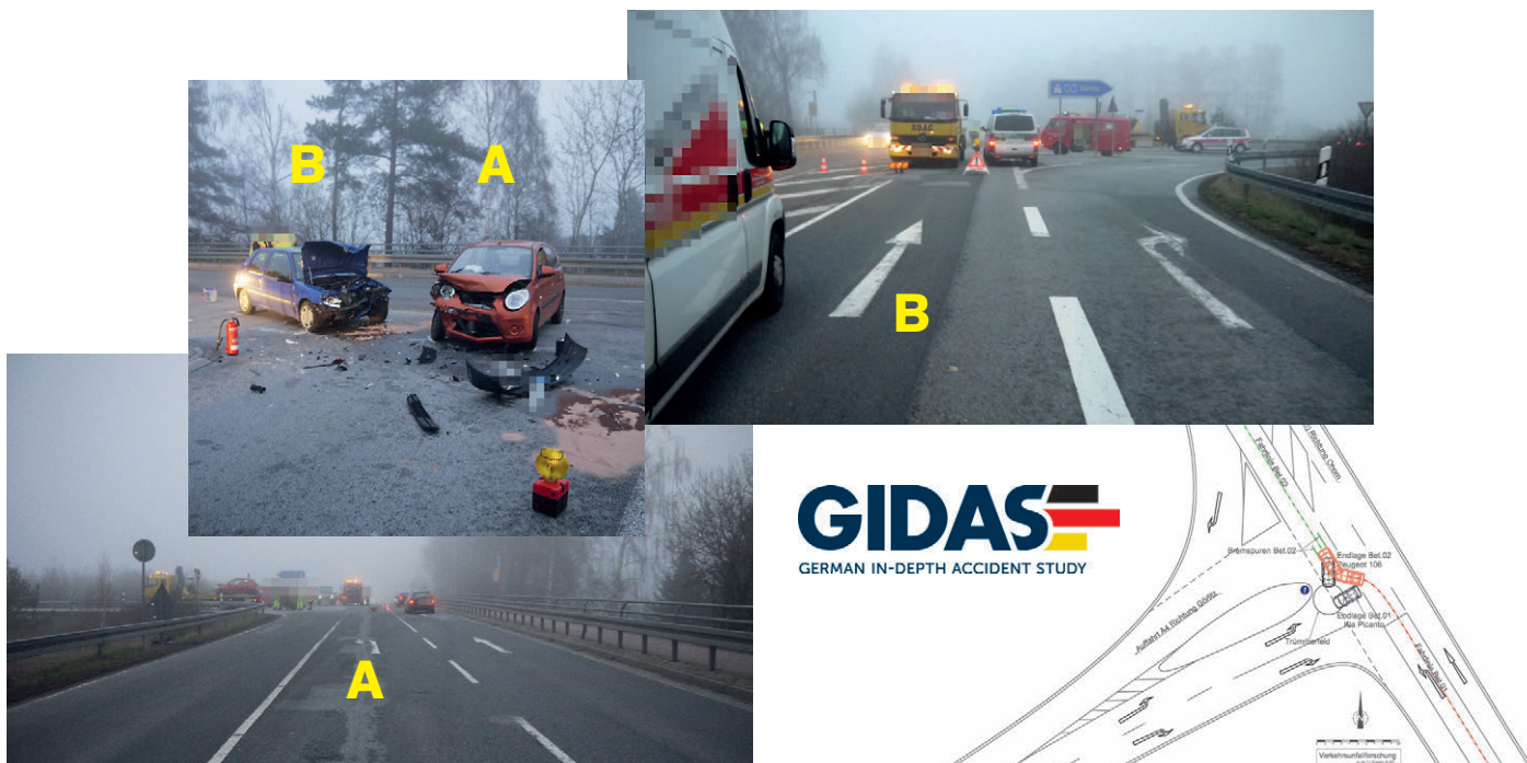
A GIDAS example case that was analysed in-depth in view of traffic accidents between 2 passenger cars at intersections – vehicle A: Turning vehicle and vehicle B: Vehicle with right of way
