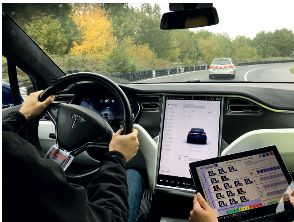
The tablet tool can be used in the future to evaluate the safety of man-machine interaction in series production vehicles in studies with test drivers on proving grounds
