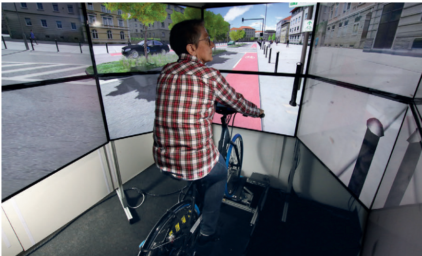
BASt's bicycle simulator (photo: Guido Rosemann, BASt)
