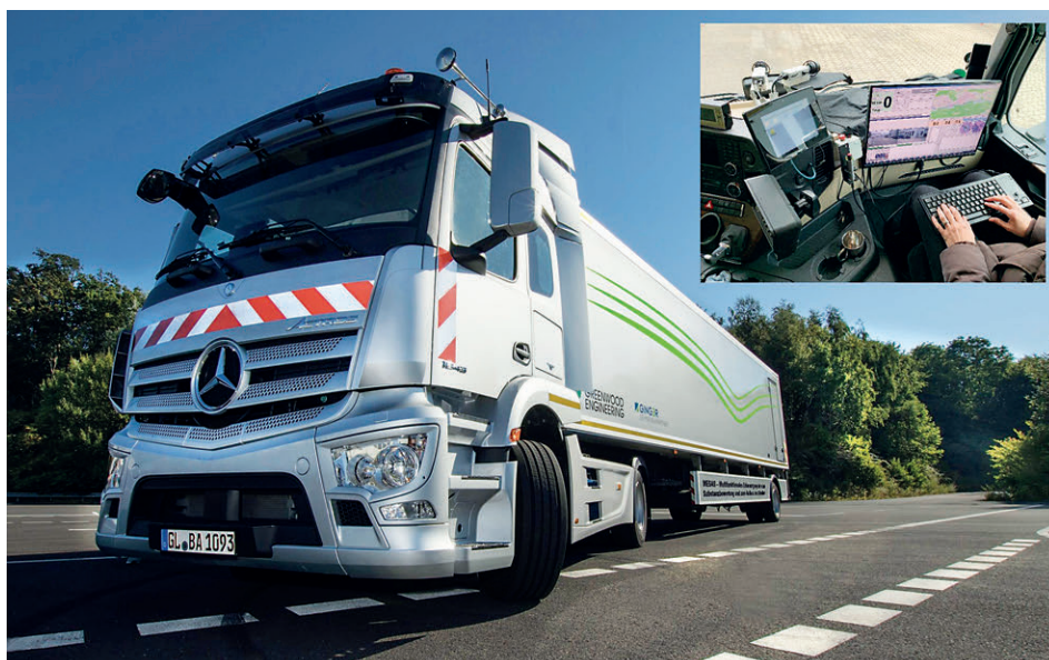
MESAS measurement vehicle and the operator's work station inside the driver's cabin
