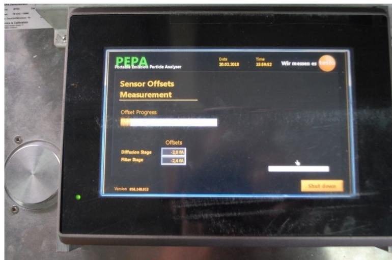
Abbildung 2.3.3: testo PEPA "Sensor Offsets Measurement"
