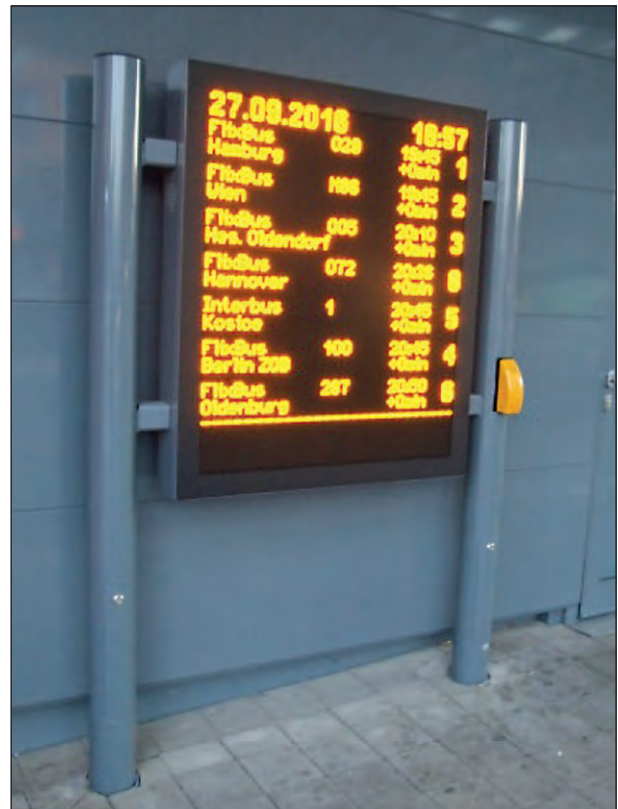
Fig. 3: Dynamic passenger information panel with demand button for speech output
