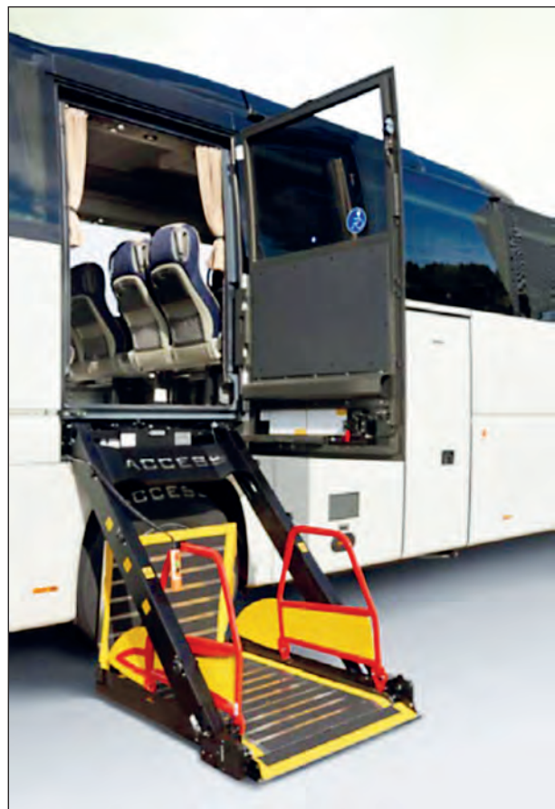
Fig. 1: Accessibility for wheelchair users to a high-deck bus with a chair lift (photo: VDL Bus & Coach)
