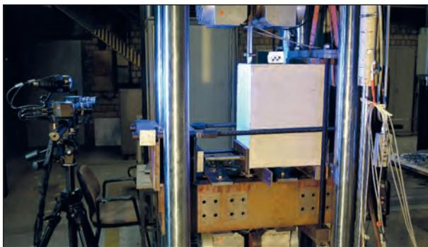
Fig. 2: Specimen (BEc20b) in the test set-up (load applied vertically)
