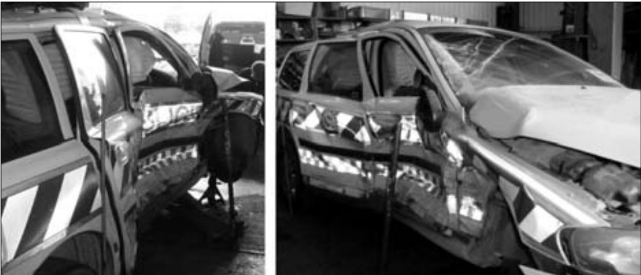
Figure 1: Case 1 – side impact damage
