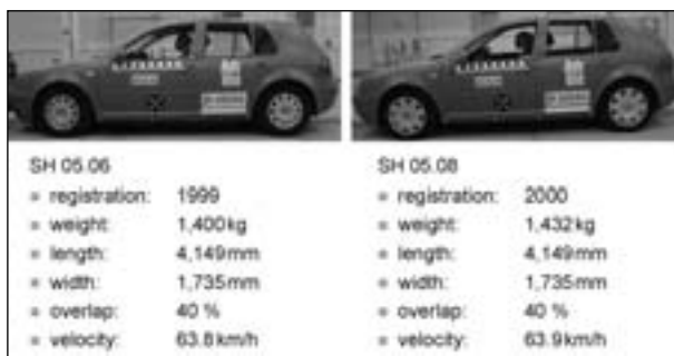
Figure 3: Test vehicles: used VW Golfs IV
