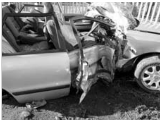
Figure 3: Case 2 – side impact damage
