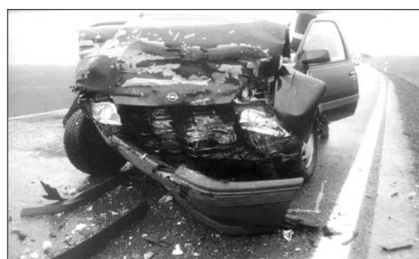
Fig. 6: Frontal crash (car of compact class type, main impulse direction from 12h)
