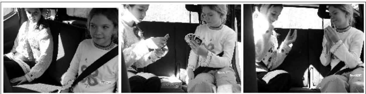
Fig. 6: Correct position of the 3-point belts, inappropriate plant of 3-point belts “playing children”
