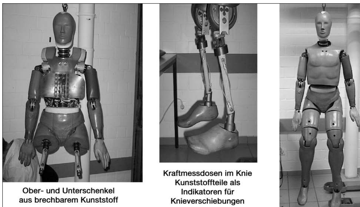
Bild 4.22: Motorcyclist Anthropometric Test Device MATD
