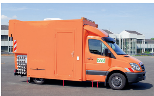
Methods to detect longitudinal unevenness: MEFA (multi-functional detection system for road surface analysis) (left) and planograph (right)
