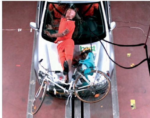
Left: Cyclist dummy for testing emergency braking systems
