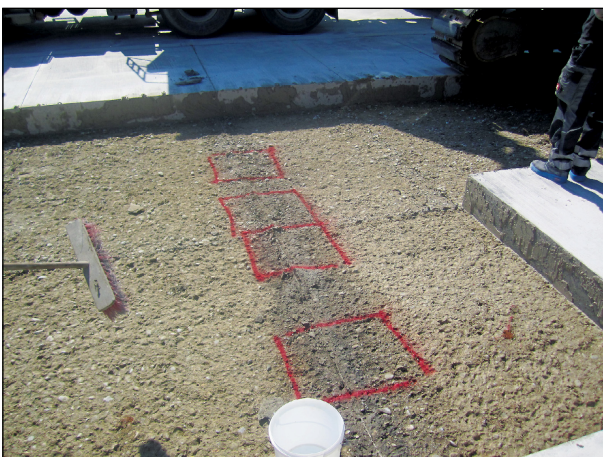
Fig. 4: Surface of the modified gravel base layer KTS in the joint area, the points of withdrawal are marked in red
