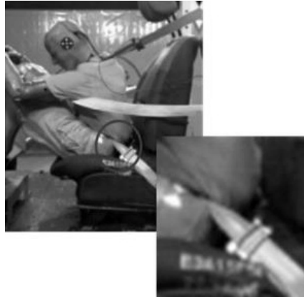
Figure 6. Illustration of the submarining phenomena during a frontal impact
