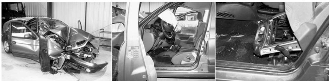
Figure 7. Real case: frontal impact at 65km/h against a tree, with a driver having an AIS4 injuries at abdominal region (dilacerations of abdominal muscles and rupture of the colon). The seat-cushion of the driver is collapsed on 20cm.
