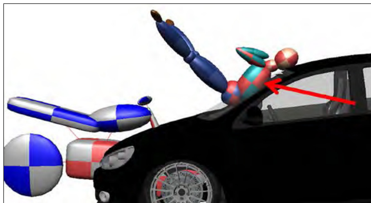
Figure 5: Typical injury mechanism of an aortic rupture for motorcyclists: Caudal or caudal-ventral thoracic load (red arrow) respectively a frontal or lateral impact of the thorax to the roof, A-pillar or side compartment of the car/truck
