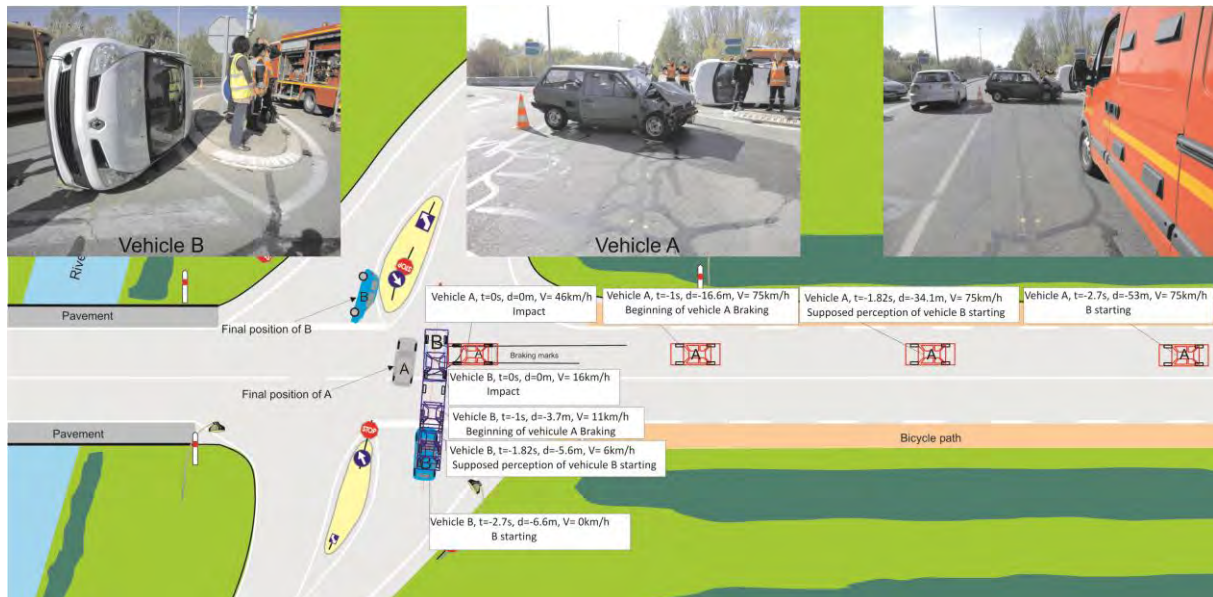
Figure 3. Results of the kinematics reconstruction, spatiotemporal description of its proceedings
