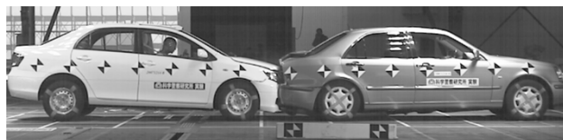
Figure 4. Physical test of rear-end collision
