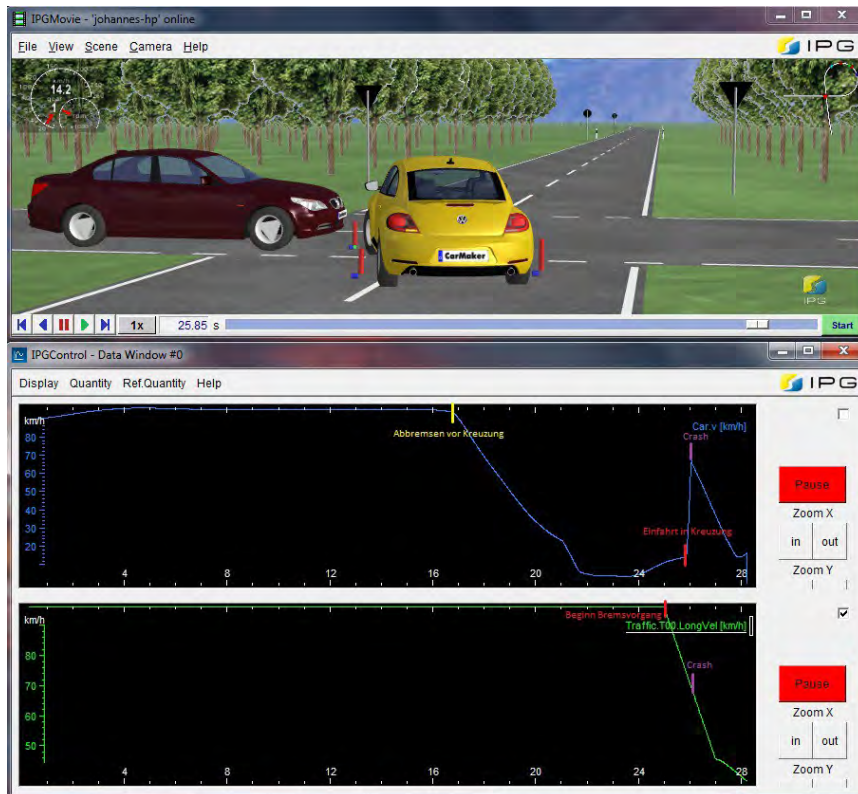
Figure 4.10: The most frequent accident joining/crossing traffic in the IPGControl data window and in IPGMovie
