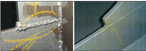
Fig. 3: Hochstraße A Leverkusen (A1); left: crack in the weld between vertical and horizontal stiffener(1994); right: crack in the TS of the bottom plate (2006)
