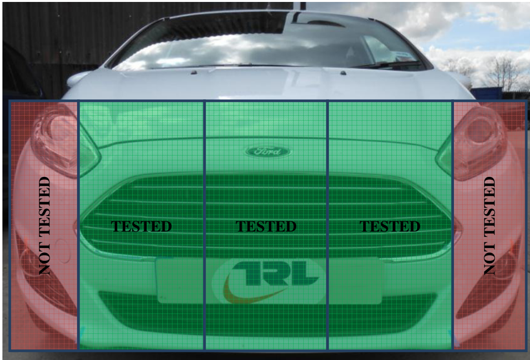
Figure 1. Bumper tests are divided into thirds for three tests
