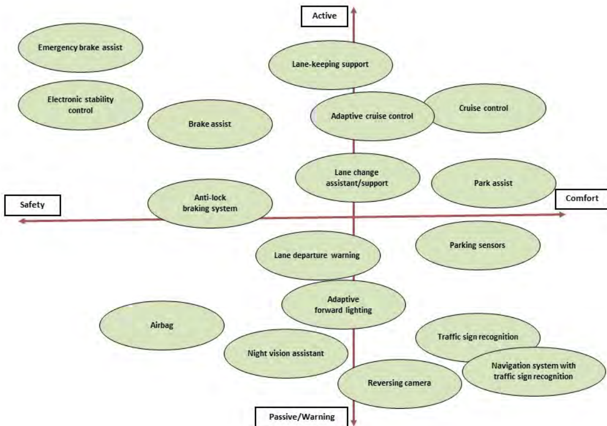
Fig. 16: Functions and degree of support of driver assistance systems (based on BANDMANN, 2008)
