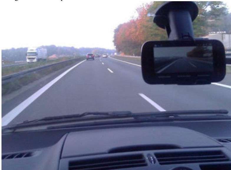
Figure 2. Setup for investigation of naturalistic driving data using smartphones.
