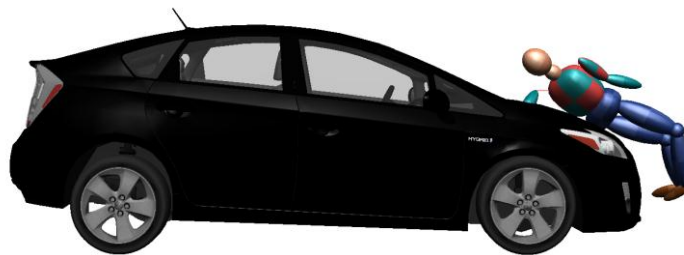
Figure 2. Kinematics of pedestrian; Contact phase (Scoop up)
