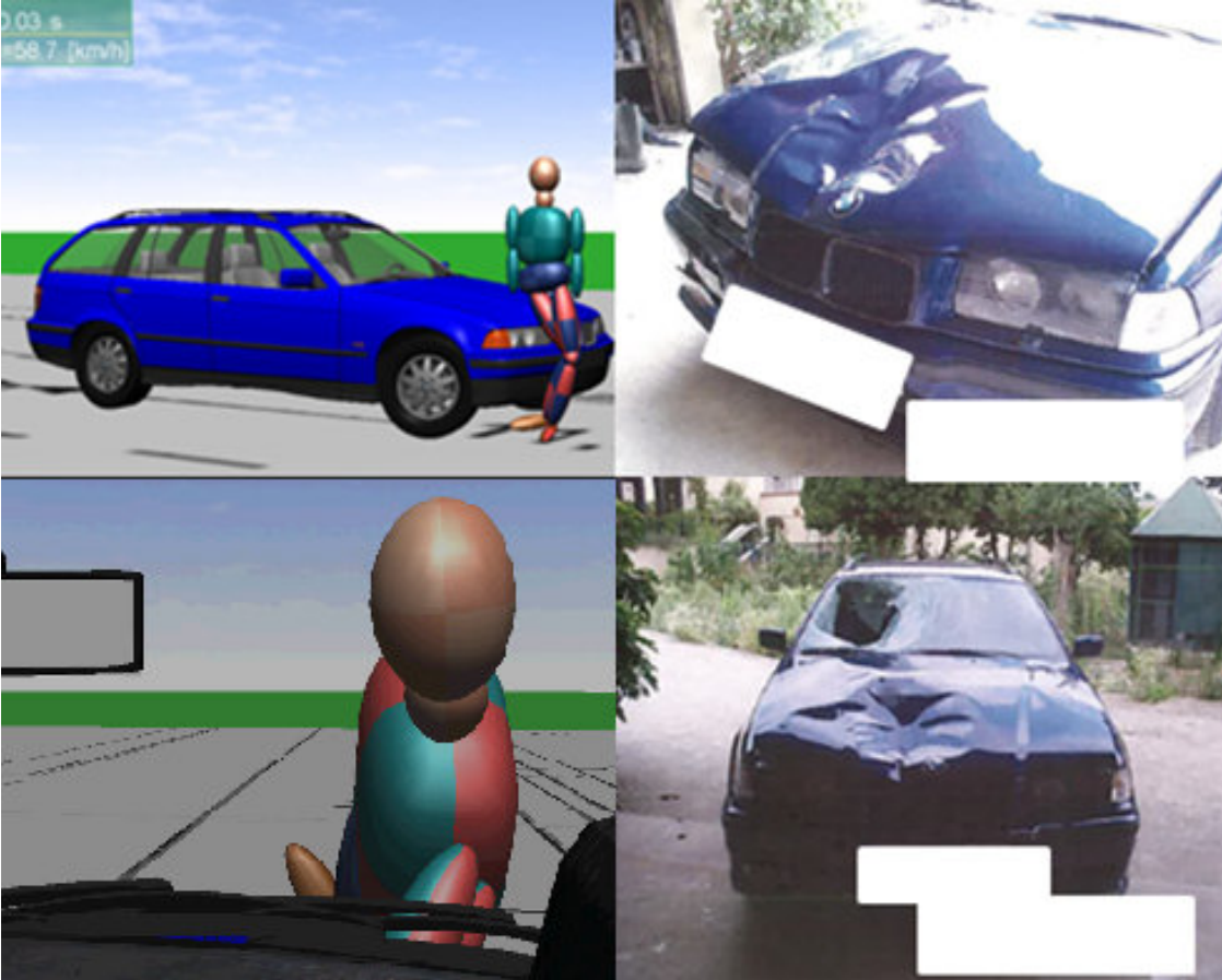
Figure 5. Compatibility between injuries and structural deformation.
