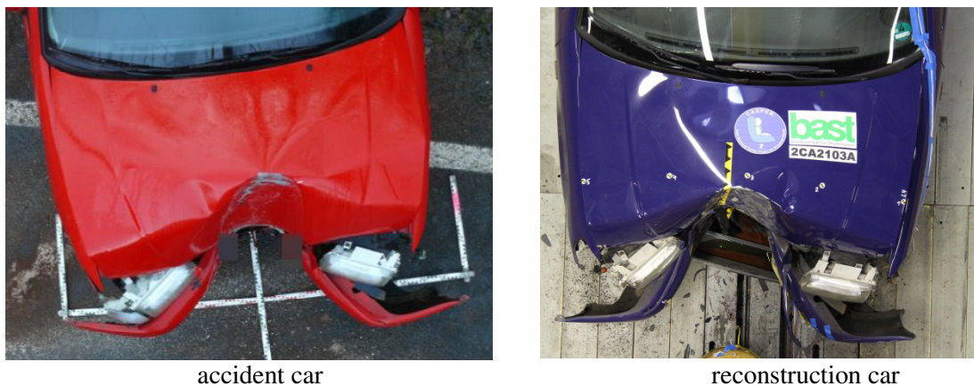
Figure 6: Comparison of vehicle damage between accident and accident reconstruction Accident 2
